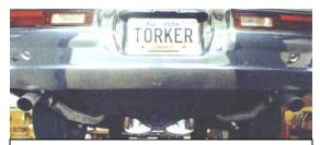
Notice bottom of mufflers are just below the heighth of the bottom of the differential.
