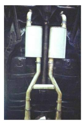
for proper fit, then begin "fine tuning" the overall fit of the system. Do not tighten clamps until you have everything fitting. Consider suspension movement while fine-tuning.
